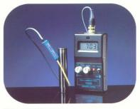
**GAUSS METERS measure the magnetic strength** of the magnets
